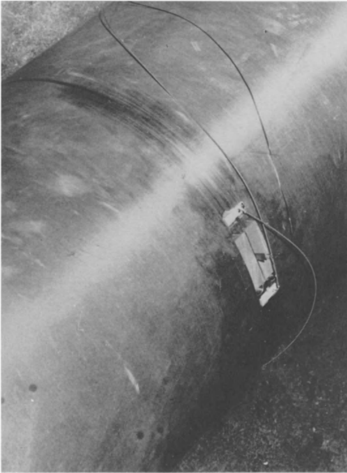
Fig. 18. Intermediate bar of M = 390 kg with the piezoelectric ceramics mounted in a slot which contracts at low temperature, providing a very good coupling.
